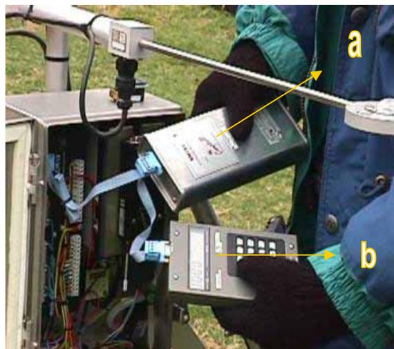
Figura.6. (a) keypack, (b) storage module
